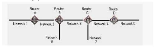
Router C uses RIP and has split horizon enabled. Which cost metric does Router C advertise on Netwok 3 regarding Network 6?
