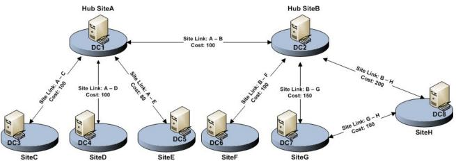
The Bridge all site links option is enabled. You need to ensure that domain controllers in the spoke sites can replicate with domain controllers in only the hub sites. The solution must ensure that domain controllers can replicate if a server fails in one of the hub sites.
