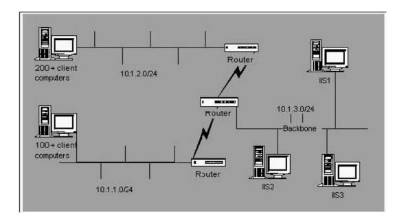
A. Configure one DNS server so that it has one DNS zone. Enable Round Robin. Create an A (host) record for appz for each Web server's IP address.
