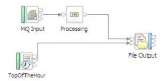
It is expected the previous file will be removed before the next file is written in its place. If this has not happened, what are the options available to the solution developer on the File Output node?
