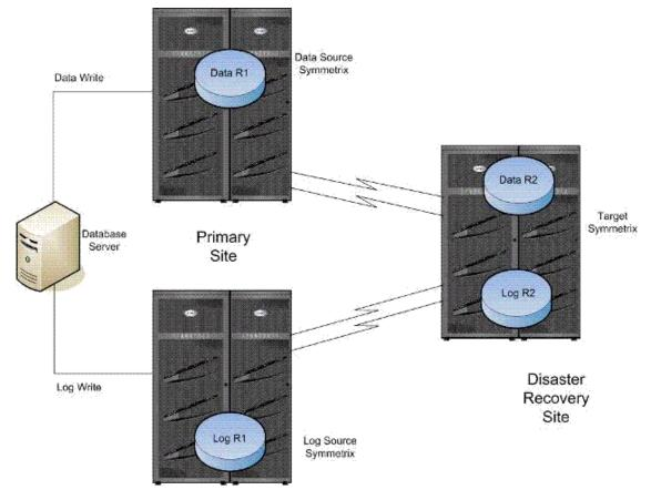
A. An SRDF failover would be initiated on all volumes and processing would automatically be switched over to the disaster recovery Site.
