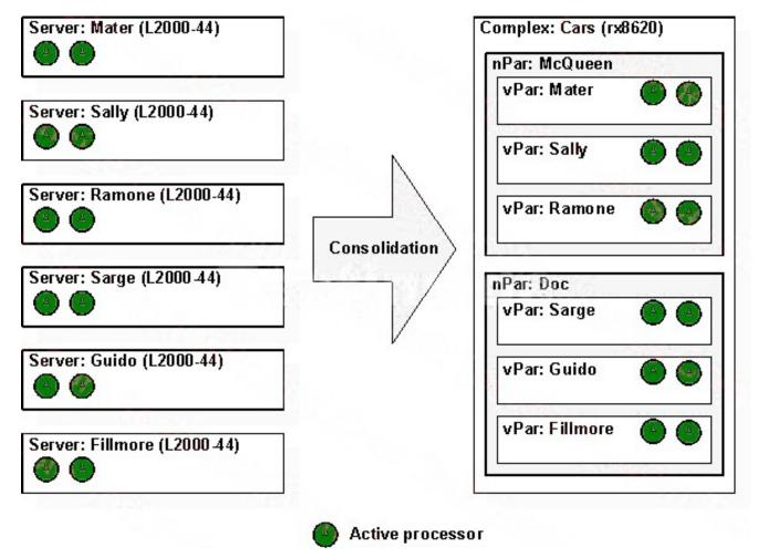
A customer has consolidated six L2000 servers to Virtual Partitions in an rx8620 as shown in the diagram.
