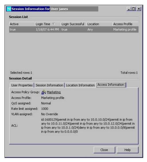
A.The user received an IP address in the range of 10.0.10.0/24.
