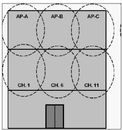
A.AP-A: channel 1, AP-B: channel 6 and AP-C: channel 11 B.AP-A: channel 7, AP-B: channel 8 and AP-C: channel 9 C.AP-A: channel 11, AP-B: channel 1 and AP-C: channel 6 D.AP-A: channel 2, AP-B: channel 3 and AP-C: channel 4
