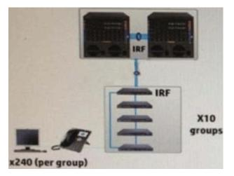
A network architect is planning a voice over IP (VoIP) solution for a customer. A computer connects to each VoIP phone, which is Link Layer Discovery Protocol Media Extensions (LLDPMED) capable and supports 802.1X. The Phone then connects to the Ethernet jack. The design currently calls for edge ports to enforce 802.1 xs to a wireless Network Policy Server (NPS), and RADIUS policies assign users to VLANs based on their identity.
