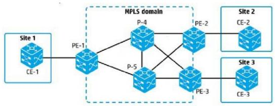
An MPLS VPLS solution (non-hierarchical) will connect the sites shown in the exhibit Which pseudo wire (PW) connections must the administrator configure?
