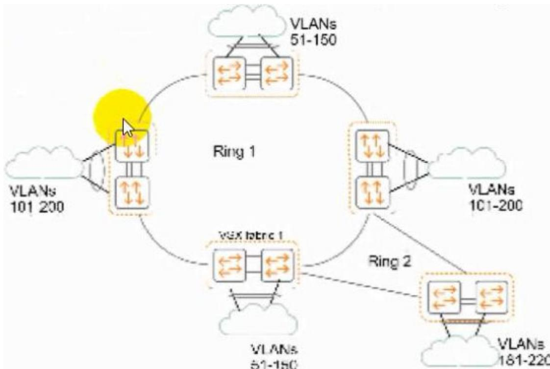
which shows the topology for an Ethernet Ring Protection Switching (ERPS) solution.
