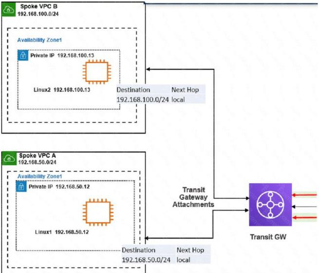
The exhibit shows a customer deployment of two Linux instances and their main routing table in Amazon Web Services (AWS). The customer also created a Transit Gateway (TGW) and two attachments Which two steps are required to route traffic from Linux instances to the TGWQ (Choose two.) A. In the TGW route table, add route propagation to 192.168.0 0/16
