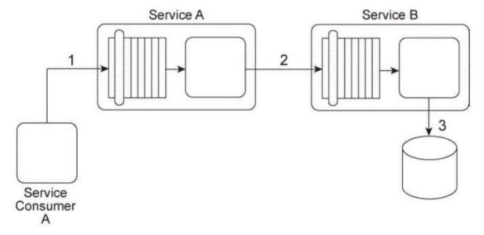
A.The Data Model Transformation pattern can be applied so that the invoice document sent by Service Consumer A is transformed into an invoice document that is compliant with the XML Schema B used by
