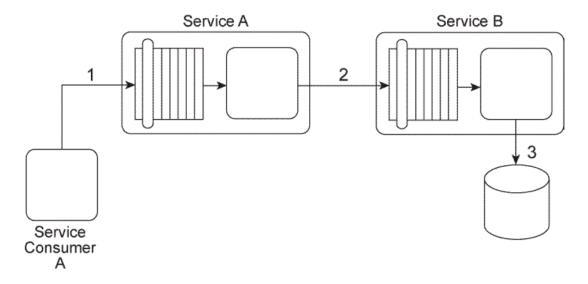
A.Service Consumer A can be redesigned to use XML Schema B so that the SOAP message it sends is compliant with the service contract of Service A. The Data Model Transformation pattern can then be applied to transform the SOAP message sent by Service A so that it conforms to the XML Schema A used by Service B. The Standardized Service Contract principle must then be applied to Service B and Service Consumer A so that the invoice XML document is optimized to avoid unnecessary validation.
