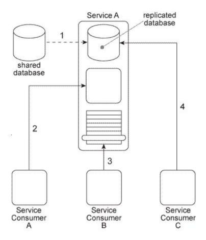
A.The Contract Centralization pattern can be applied to force all service consumers to access the Service A architecture via its published service contract. This will prevent negative forms of coupling that could lead to problems when the database is replaced. The Service Abstraction principle can then be applied to hide underlying service implementation details so that future service consumers cannot be designed to access any part of the underlying service implementation.
