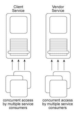
A.The Rules Centralization pattern can be applied by extracting the business rule logic from the Client and Vendor services and placing it into a new Rules service. This will naturally improve the runtime performance of the Client and Vendor services because they will no longer be subjected to the high concurrent access of service consumers that require access to the business rules logic.
